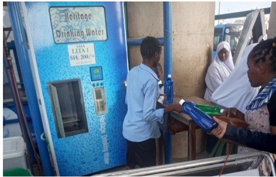
Figure 11 Showing Uncovered Dispensing Nozzles at Sampling Point
