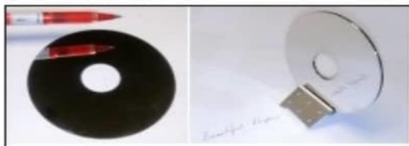
Two Photographs Showing the Reflection Standard
