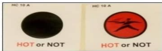
Photograph of the Food-box Label Thermochromic Film Used
